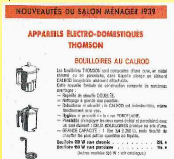
1939 Calrod heating elements made of Stainless Steel (Ultimheat Museum document)
